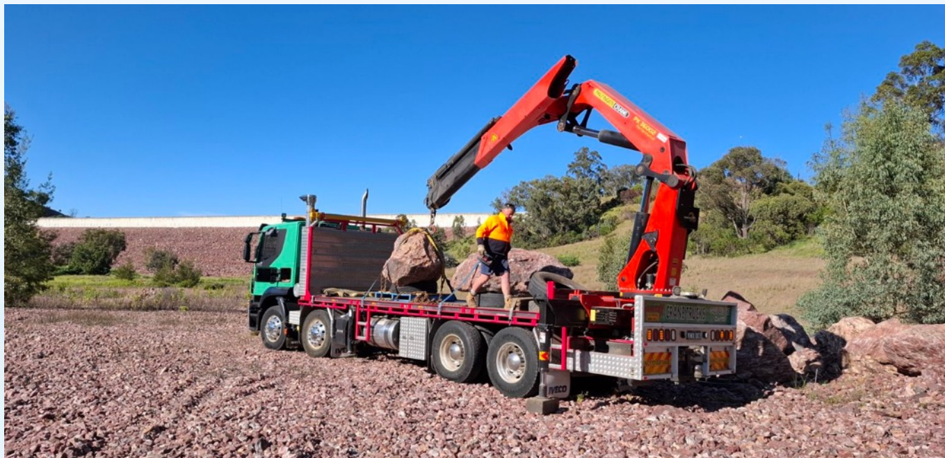
Uplift and loading of two chert boulders of approximately four tonnes. The white wall in the background is the top of Chaffey Dam. Image courtesy M. Smith.
